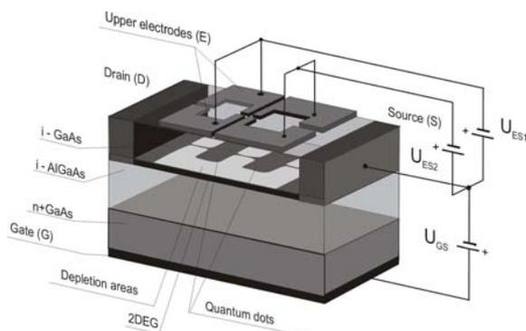
Fig. 1. The structure of two coupled quantum dots.
