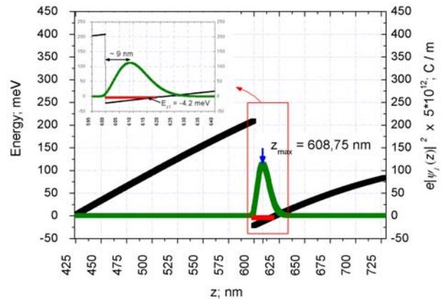
Fig. 3. Quantum well formed at the GaAs/AlGaAs interface (black line and left axis). Energy of the ground state  $E_{z1}$  (red line) and corresponding wave function  $\psi_1(z)$  (green line and right axis). The inset shows the neighbourhood of the heterojunction.
