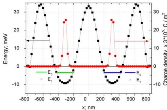
Fig. 5. Cross-sections of charge density (red circles) and potential distribution (black squares) after self-consistent procedure, performed in  $xy$  plane. There are also energy levels  $E_0, E_1$  marked in each quantum well.
